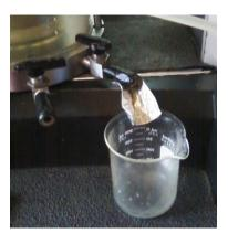
21) Topping off & purging the cell: Inevitably, some water will be lost while preparing the triaxial cell for testing. The
