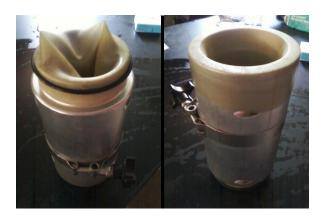
8) Place two pieces of 7.0cm diameter **filter paper** on top of the bottom cap. With a paintbrush, apply a dusting of baby powder to the inside of the membrane.
