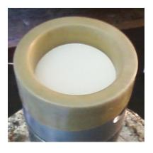
13) Apply a thin film of vacuum grease to the **top cap**. Clear dirt from inside the top of the membrane – a slightly damp paper towel works well. Press the top cap into the remaining space at the top of the mold.
