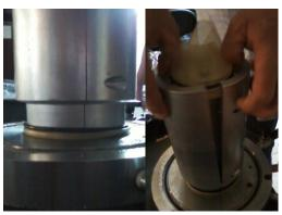
15) Apply vacuum grease liberally to bottom of **Plexiglas** shell and to bottom large o-ring. Place onto **triaxial cell** base. Close all the valves on base except for the one furthest to the right and fill the cell to about 2 inches from the top with tap water. Clean off the top of the Plexiglas shell and apply vacuum grease.
