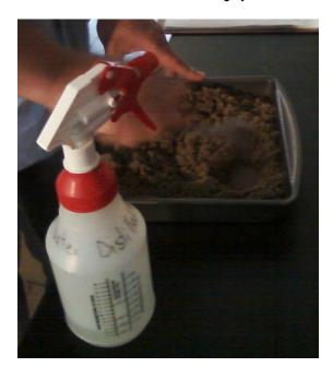
5) Record the new mass of the sample and container as "Container Start Weight". Cover with **plastic wrap** to contain moisture as necessary.
