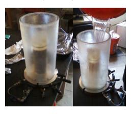
16) Lift the pusher rod of the **triaxial cell cap**, and confirm that it will fall under its own weight. Confirm that the large o-ring is sitting inside the groove the triaxial cell cap. Put the pusher rod into the top cap of the specimen and lower the triaxial cell cap onto the Plexiglas shell. If running a test at a temperature other than ambient, make sure to use the cap with a copper coil.
