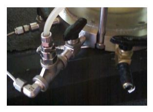
22) Confining Pressure: A complete set of triaxial test data consists of tests run at four different confining pressures (5, 10, 15, 20 psi). Dial the regulator to until the pressure inside the triaxial cell is correct. Be patient and make sure that the pressure is correct and not changing before starting the test.
